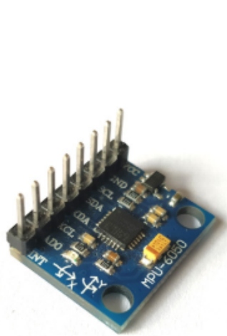
(a) IMU BreakoutBoard [43] (b) MPU6050 Functional Block Diagram Board [44]
